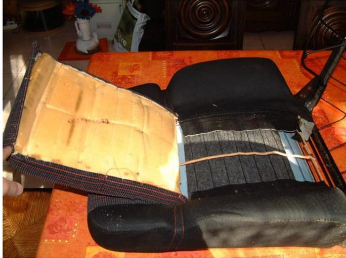
Our attention now moves to the side bolster attachment rings. To get to these, fold the middle section back out of the way, then lift the side section extension wings back.
