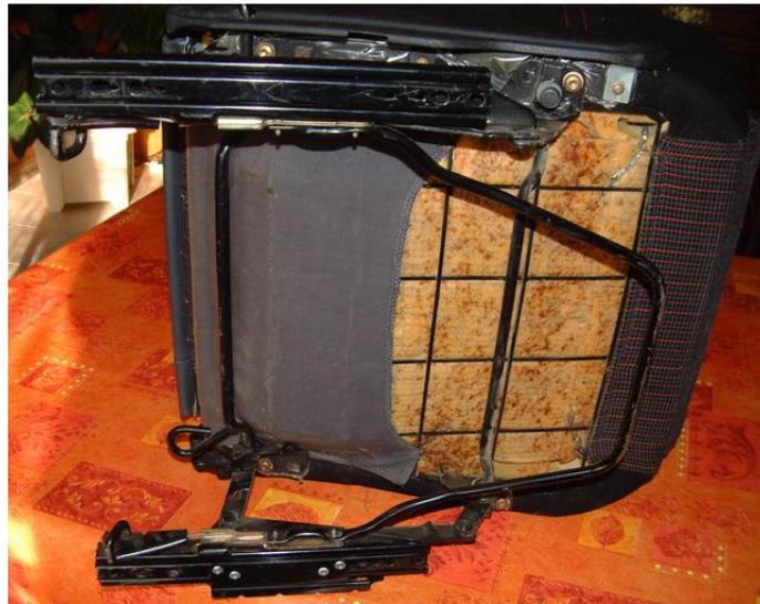
With the seat as above remove the plastic outer trim piece (3 Philips screws) and then take off the seat runner – 4 Torx screws ( 2 per side).
