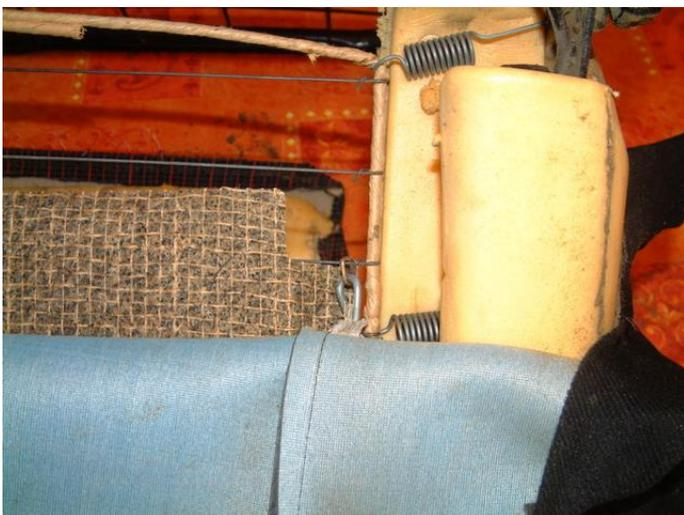
Next we tackle the back vinyl attachments; these are down each side and across the top of the middle part of the backrest vinyl section. Work from bottom to the top of the seat as shown below.
