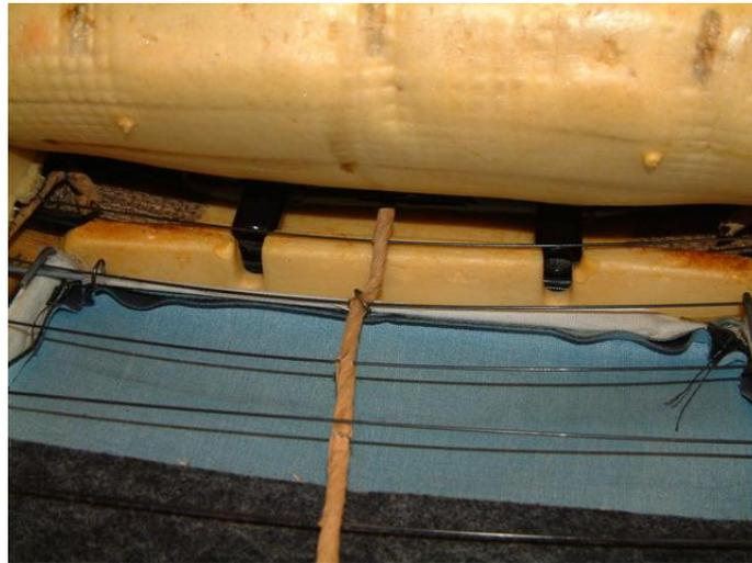
Once the vinyl is released, then we finally detach the insert itself from the centre foam section by removing the hog rings, taking care not to rip chunks of foam out as you do this. Go up each side first.
